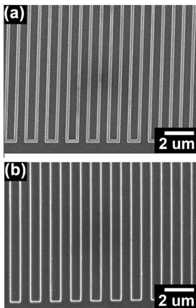
**Fig. 5.** SEM images demonstrating pattern transfer by NIL. (a) 166 nm features transferred from the Si master in Fig. 4a. (b) 39 nm features transferred from the oxidized master in Fig. 4d.
