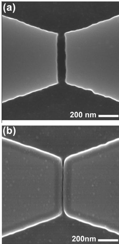
**Fig. 2.** SEM images of master features resized through oxidation. (a) A 74 nm gap in a Si master formed by EBL. (b) After growing a 55 nm thermal oxide on the Si, the 74 nm gap is reduced to 10 nm.
