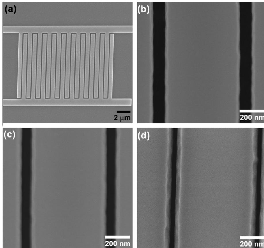
**Fig. 4.** Oxidation of an interdigitated array NIL master. (a) Original unoxidized interdigitated array master with 500 nm line widths and 166 nm gaps. The gaps are reduced to 99 nm (b), 76 nm (c), and 39 nm (d) through successive thermal oxidation processes.
