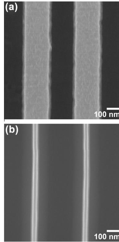
**Fig. 3.** SEM images of Si master features resized through thermal oxidation. (a) Unoxidized 226 nm Si lines fabricated by EBL. These lines were oxidized to a width of 356 nm (not shown) and then, (b) etched in BOE to remove the  $\text{SiO}_2$  layer producing the 55 nm wide Si lines shown.
